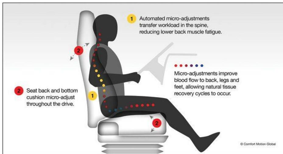
*CMG's customizable algorithm, a first of its kind technology, can be programmed into any memory seat and can additionally actuate any other system in the seat such as lumbar support, bolsters, heating and cooling, and existing massage functions.*
